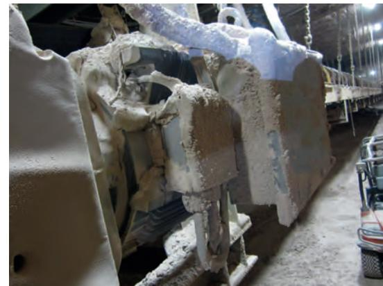
*The drive system supplied by Synergy Engineering in conjunction with Nidec needed to be capable of starting the conveyor 35 times per hour and of operating 20 hours a day, 350 days a year in challenging conditions such as potash dust accumulation on the motor*
